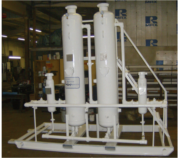
Dual tower desiccant skid with filters
