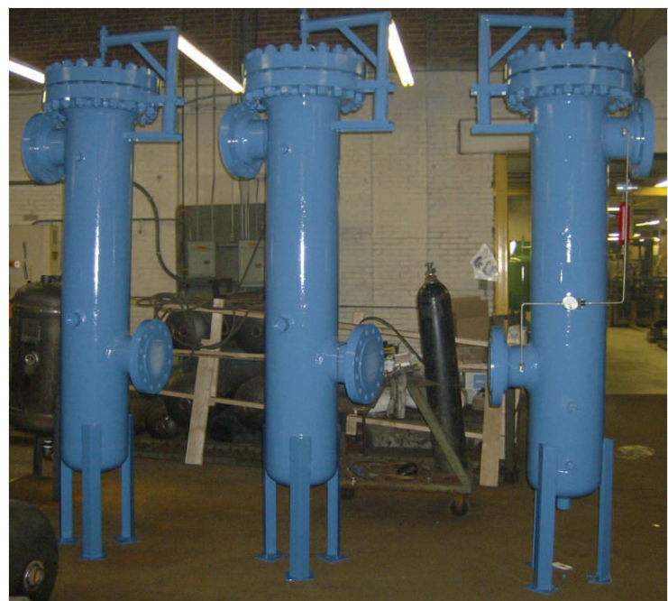
1440 psig filters for Marcellus gas compressor station
