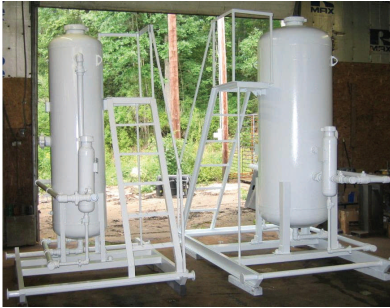
Multiple desiccant skids
