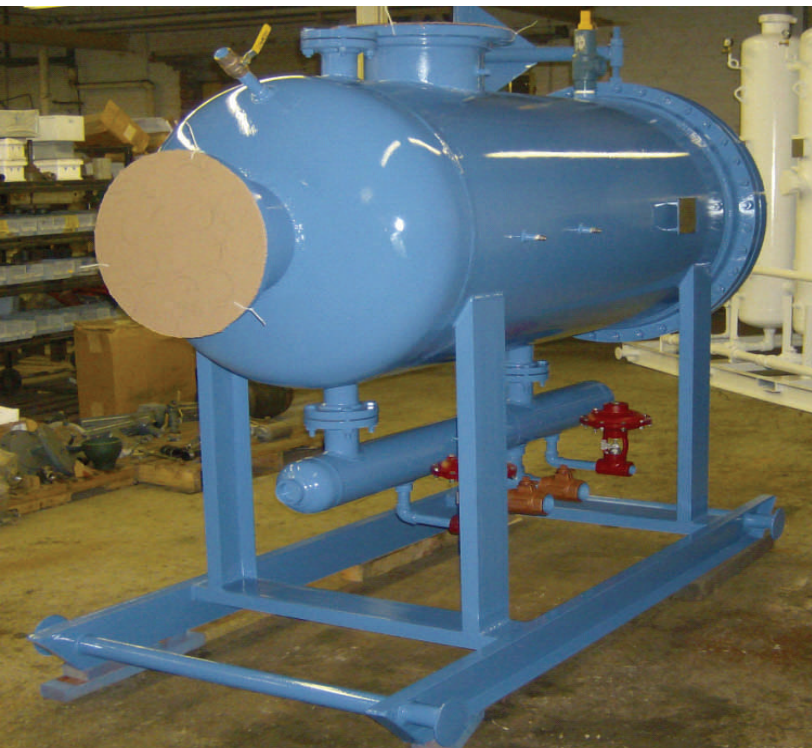
25 mmsfd coalescing filter with dump tank
