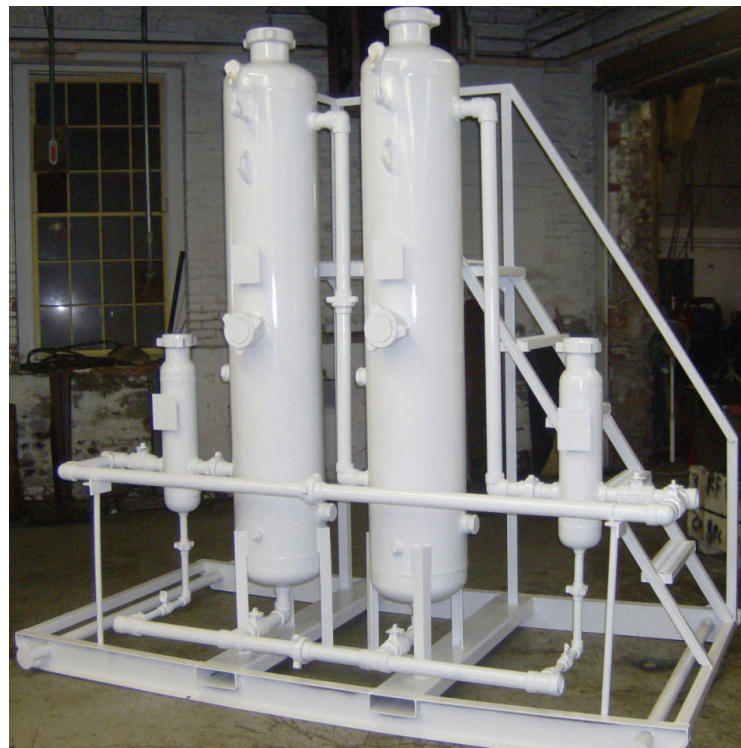
Gas desiccant skid with filters
