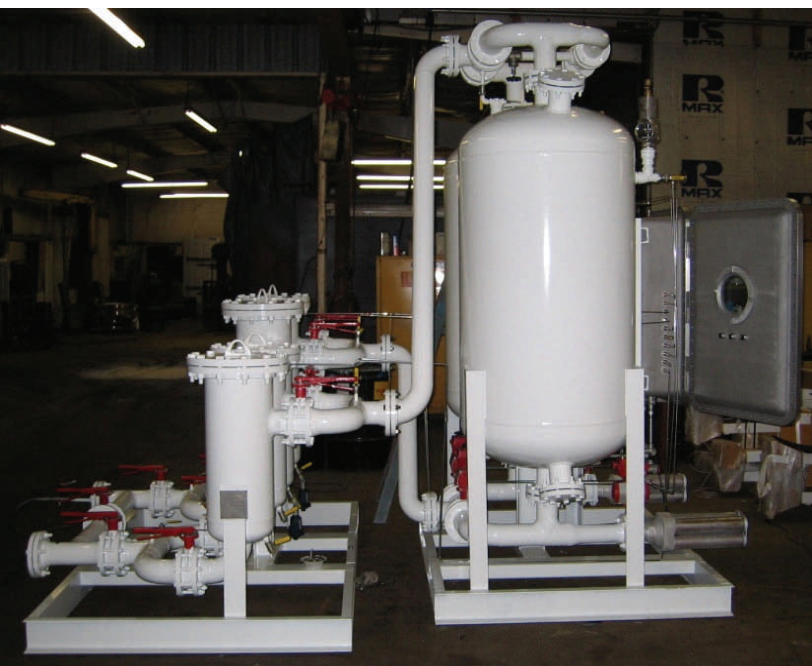
Explosion proof PSA desiccant skid with filters
