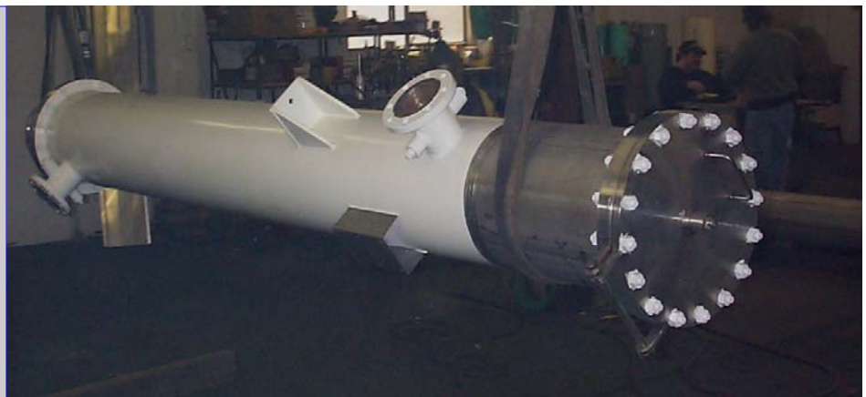
TEMA type BKU; Shell Side: 500psi/400F, Tube Side: 400psi/400F, Double T/S's, Shell inlet designed to support 10,000lbs, Vacuum dried to a dew point of -20F & then purged w/Nitrogen to 3-5psi for shipment/storage.
