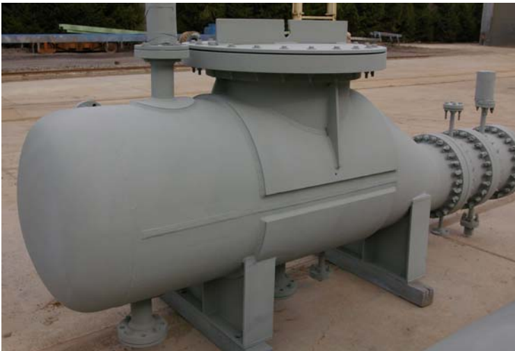
TEMA type BKU; Shell Side: 500psi/400F, Tube Side: 400psi/400F, Double T/S's, Shell inlet designed to support 10,000lbs, Vacuum dried to a dew point of -20F & then purged w/Nitrogen to 3-5psi for shipment/storage.
