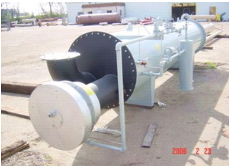
750,000 BTU Inline Heater
